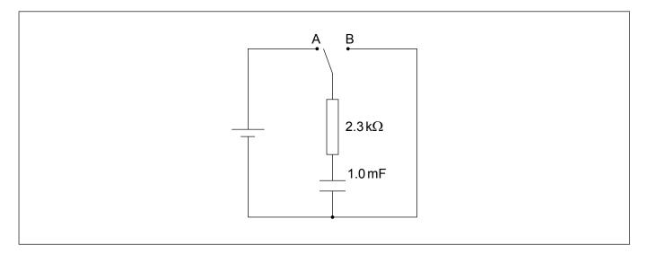
The capacitor is initially uncharged. At time t = 0 the switch is moved to position A. The initial current in the resistor is  $3.9 \,\text{mA}$ .
